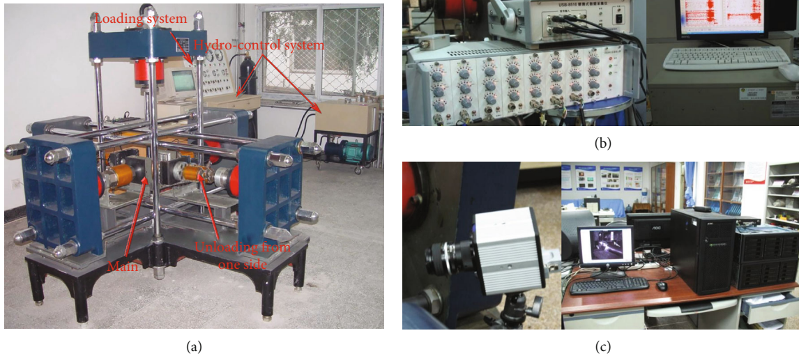
FIGURE 1: True triaxial experimental host and hydraulic control system: (a) force and deformation acquisition system; (b) acoustic emission monitoring system; (c) high-speed image recording system.
