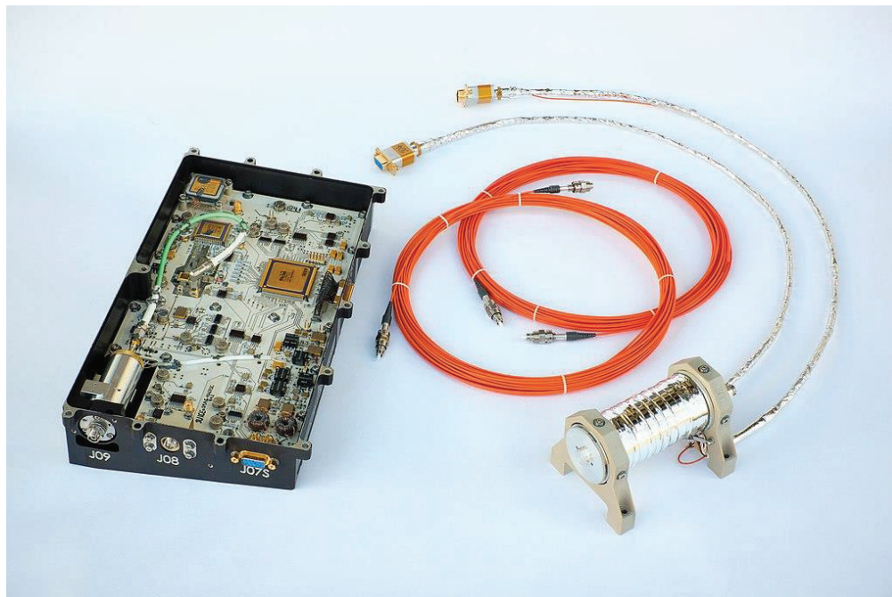
Figure 1. Flight unit of the JUICE J-MAG scalar magnetometer: electronics with laser unit (left), optical fiber assemblies (middle) and sensor (right) (Andreas Pollinger/IWF/OEAW, MAGSCA flight model , CC BY 4.0 )
