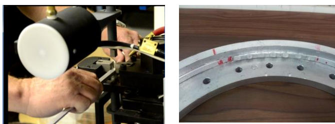
Fig. 11. (left) Ultrasonic welding machine from SonoBond; (right) TS cable ultrasonically welded for cable I_c measurement.
