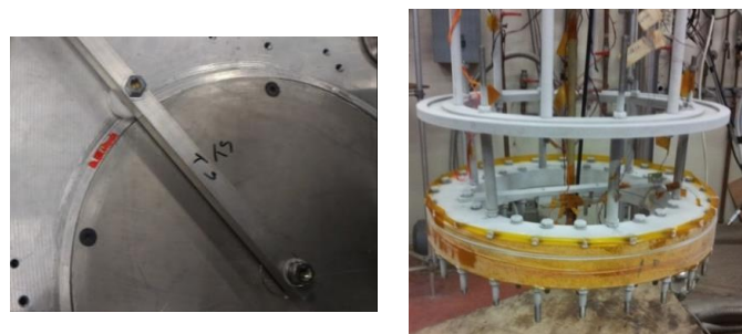
Fig. 9. (left) TS cable being assembled into sample holder; (right) TS cable ready for I_c measurement.
