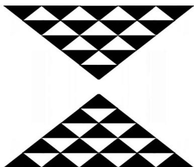
Figure 1 Construction principle of the clessidra lens composed of identical triangular prisms.
