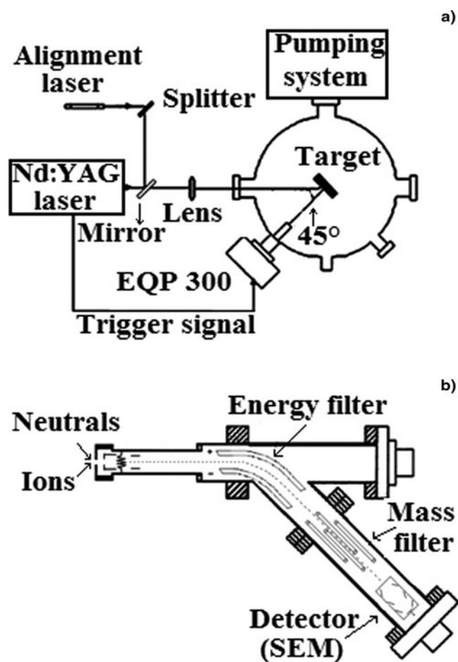
Fig. 1. The experimental setup (a) and the scheme of the EQP instrument (b).
