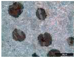
Fig. 1. Austempered ductile iron microstructure (optical micrograph 500x after polishing and 4% nital etching).
