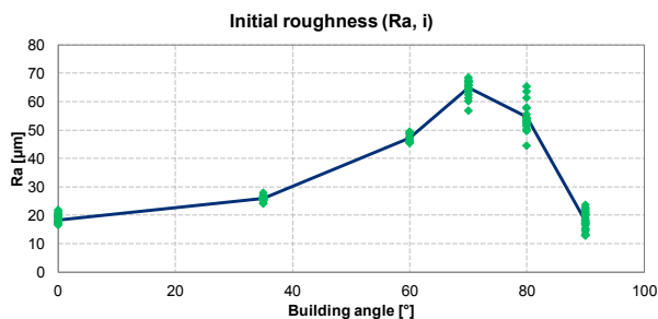
Fig. 8. Untreated samples roughness as a function of the building angle (points correspond to a single sample and the line connects the average values).
