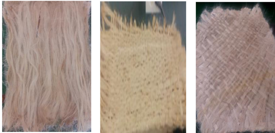
Fig. 1. Fiber Orientation a. 0^{\circ} b. (0^{\circ}, 90^{\circ}) c. \pm 45^{\circ} .
