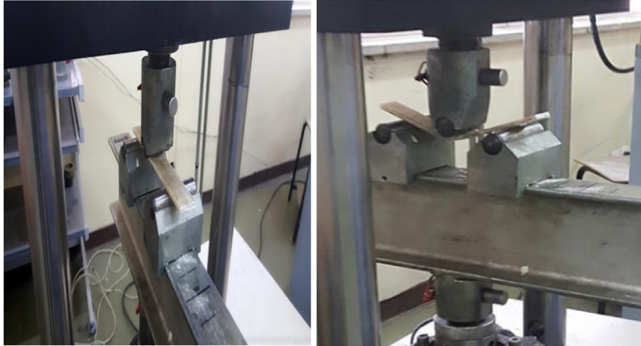
Fig. 10. Specimen under flexural testing.
