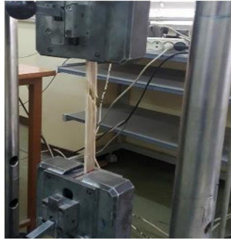
B) After failure
