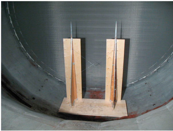
Fig. 5. Turbulence system for cable testing: Two flat wood plates are used in the settling chamber to generate low frequency turbulence.
