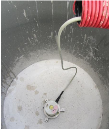
Fig.2: The sensors of Lemi18 fluxgate magnetometer.
