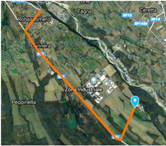
Fig. 8. Extended district heating (eDH) network layout.
