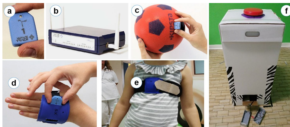
Fig. 2 a A Wavetrack sensing unit. b Wavetrack receiver. c Setup of the IMU in the ball. d IMU placed in a custom pocket on the back of the hand. e IMU in a belt attached to the chest of the subject. f Plastic enclosure to hold a Cometa Footswitch device to monitor the state of a big button (on the top of the cardboard box)
