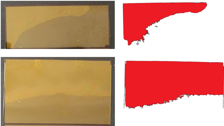
Fig. 11. Image processing applied to peeled samples. ROI (Region of Interest) original image (left) and processed image (right) for calculation of peeled area, in white. Runs reported: 100 A ( a = 10 ; e = 0 ; sample A) on top and 150C ( a = 15 ; e = 0 , sample C) on bottom.
