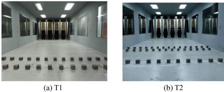
FIGURE 5 Typhoon wind-flow simulation in the wind tunnel
