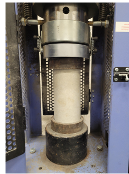
(b) Testing on 4" x 8" NSC cylinders.
