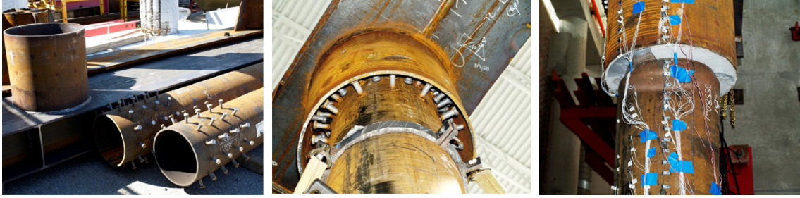
Figure 2.4: Grouted shear stud connection [41].
