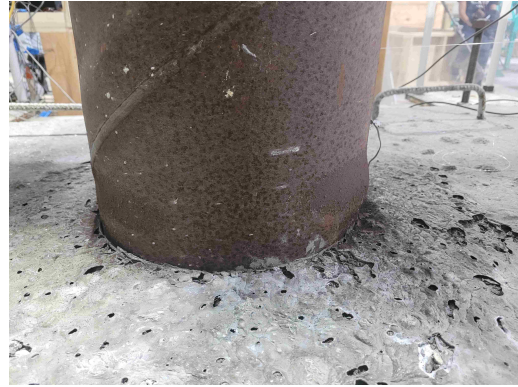
(b) Displacement level at 4\Delta_y
