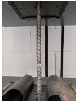
(b) Rebar fracture.
