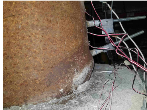
(b) Buckling of tube at 3\Delta y
