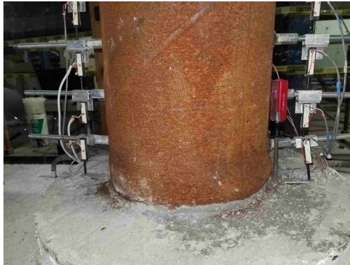
(a) Buckling of tube at 2\Delta y
