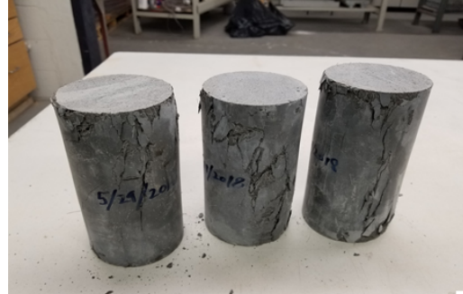
(b) Testing on 3" x 6" UHPC cylinders.
