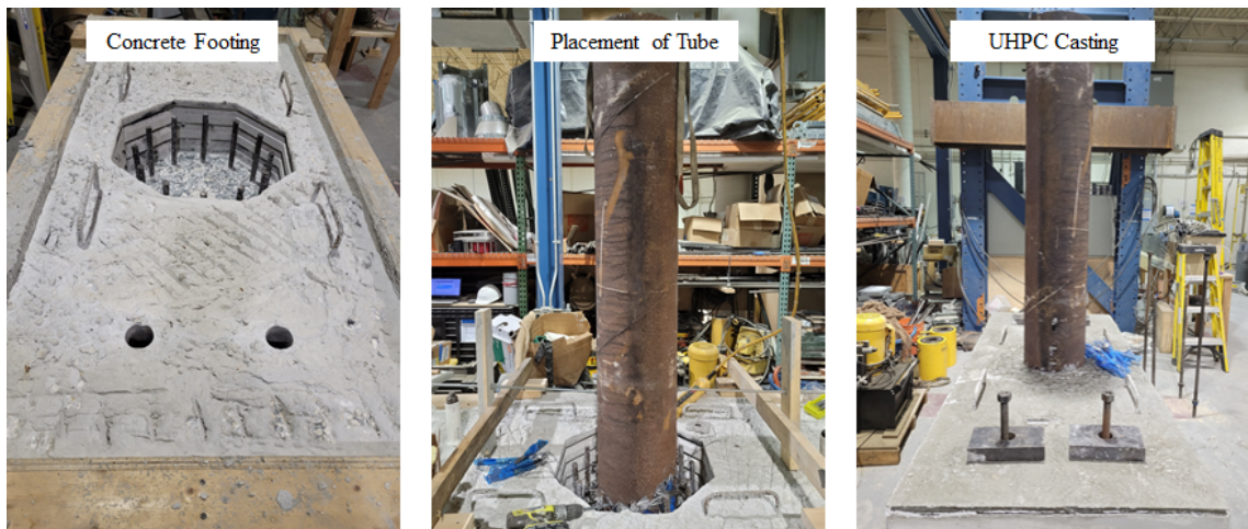
Figure 3.7: Construction of fully embedded connection (specimen-3).
