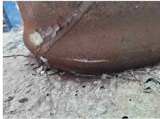
(f) Fracture in steel tube
