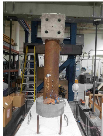
(f) Completed specimen
