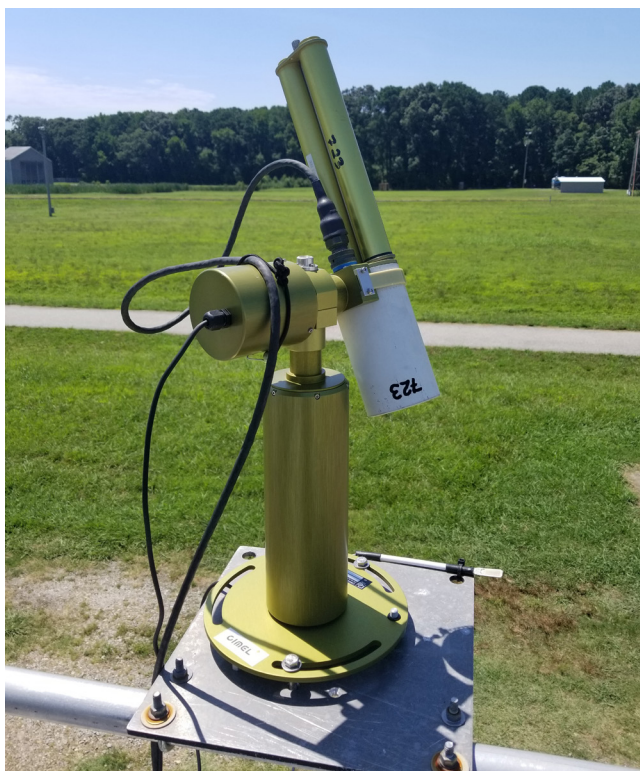
Figure 2. A Cielim sun photometer collecting aerosol data at NASA Langley Research Center. Photo taken by first author.
