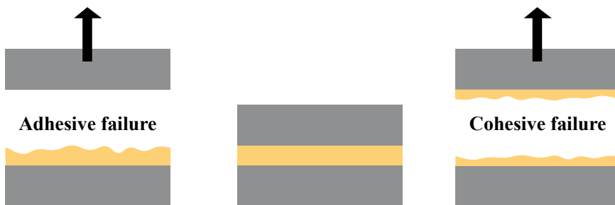
Figure 1.1 Adhesive (left) and cohesive (right) failure if two surfaces are removed from each other.
