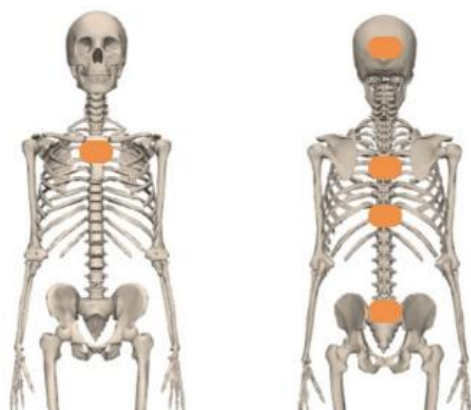
Figure 1. IMU sensors (orange rectangles) placement.
