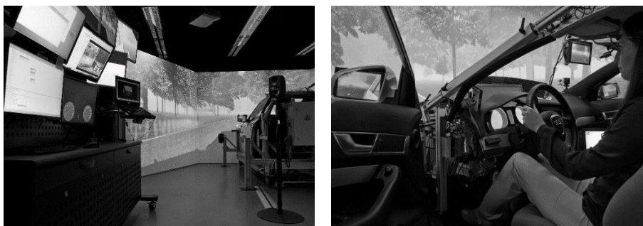
Figure 1. Driving simulator with instructor centre (left) and a participant (right)
