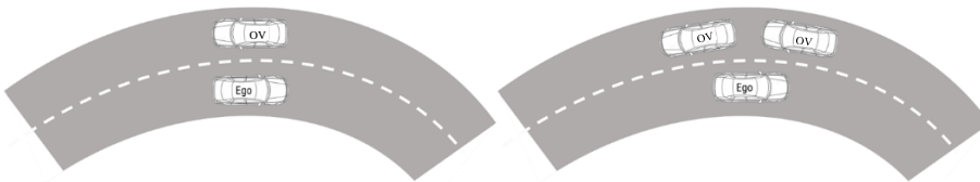
Figure 2. Ego vehicle ecountering oncoming traffic (OV) at the apex of the curve.
