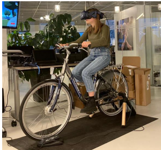
Figure 1. A bicycle simulator commonly used for traffic safety research. The bicycle is fixed to a static home trainer, the virtual reality environment is displayed on a head mounted display. Picture taken at Royal Dutch Visio rehabilitation centre.
