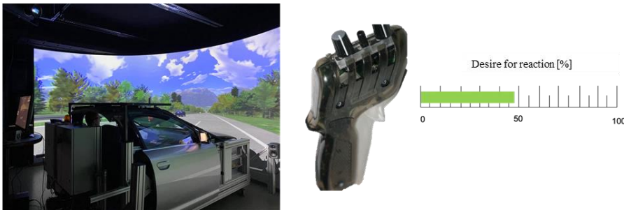
Figure 1. Driving simulator (left), handset controller with "desire for reaction" scale (right)
