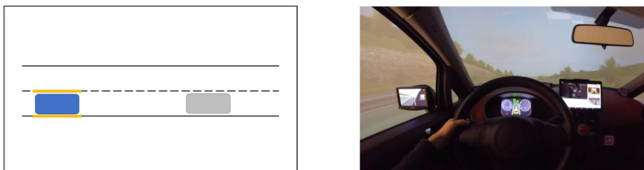
Figure 2. Exemplary screenshots of the ATS video. Schematic visualization of Lane Keeping Assist functionality (left) and video clip of ADAS activation process during driving (right).
