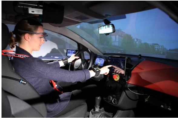
Figure 4. Experimental set-up with exemplary participant wearing eye-tracking glasses and using the tablet mounted on the middle console.
