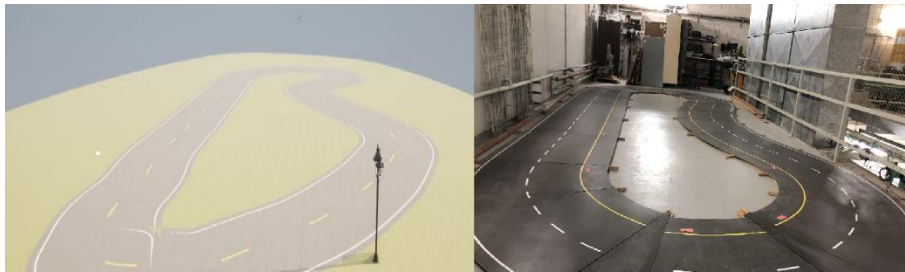
Figure 3. Driving map: CARLA (left) and the testbed (right).
