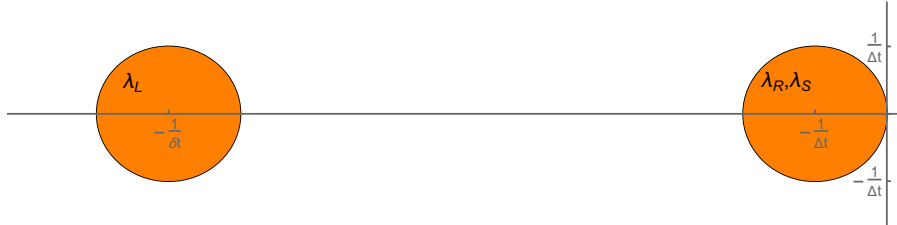
(B) Stability region of Projective Forward Euler scheme (PFE). The whole domain uses one inner time step \delta t for fast modes and one time step \Delta t for the other modes.
