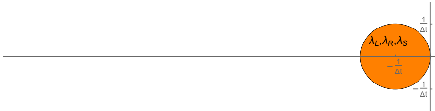
(A) Stability region of Forward Euler scheme (FE). The whole domain uses one time step \Delta t that determines the stability of all modes.
