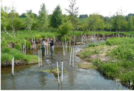
Figure 8.1 Network of mini-piezometers (PVC tubes) installed to monitor VHG and seepage fluxes in the river (photo: Daniel Käser).
