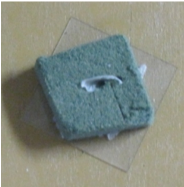
FIG. 2: Sample holder of the cross section of a fish scale.
