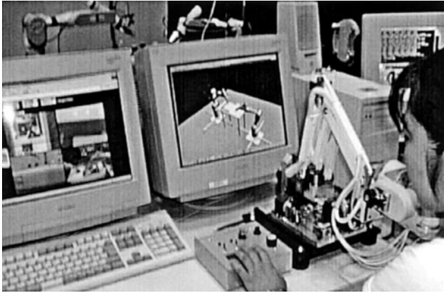
Figure 2. Local master control station.
