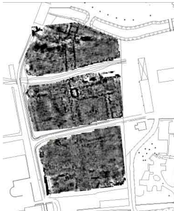
8 Gecombineerd beeld van de elektrische weerstandsmeting-en magneto metrische resultaten (© APSS & VIOE). Greyscale image of the survey results showing the integrated resistivity and magnetometer results.
