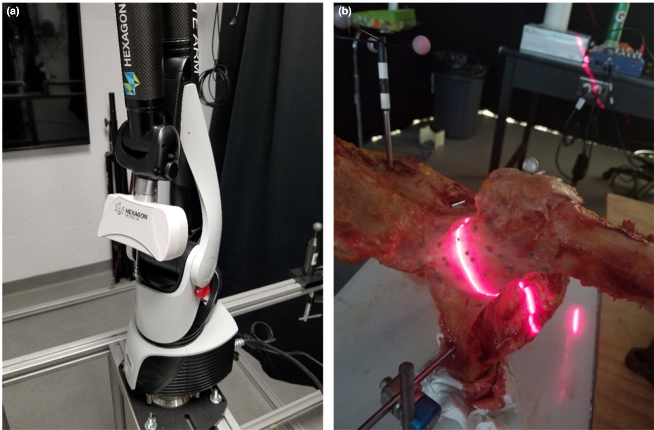
FIGURE 2 (a) Scanner mounted on the Hexagon Arm. (b) The scanning process with the scanning line.
