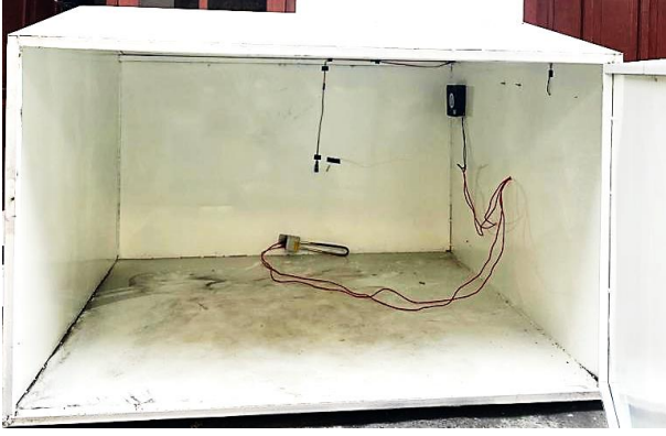
Figure 3. Placement of the DHT22 temperature and humidity sensor, heater and exhaust fan
