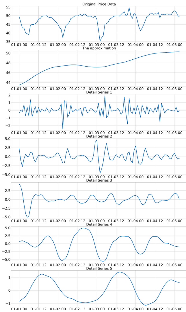
Fig. 3. Original electricity price time series and decomposed component series (time domain).
