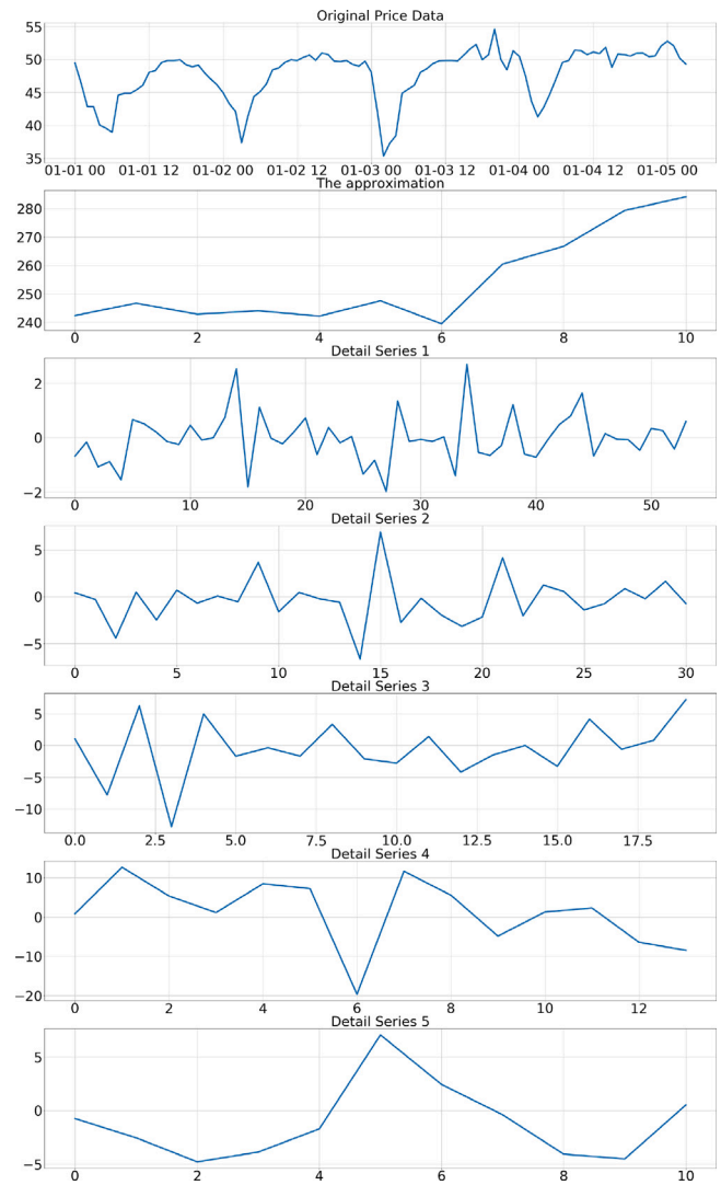
Fig. 2. Original electricity price time series and decomposed component series (frequency domain).
