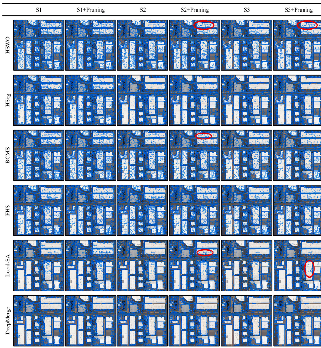
Fig. 14. The local comparison of segmentation results with and without dynamic-pruning in T4.
