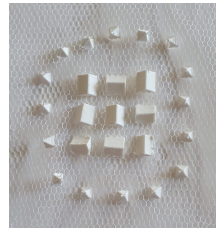
(b) Pointy texture 3D printed on textile with PLA, a non-compliant plastic.
