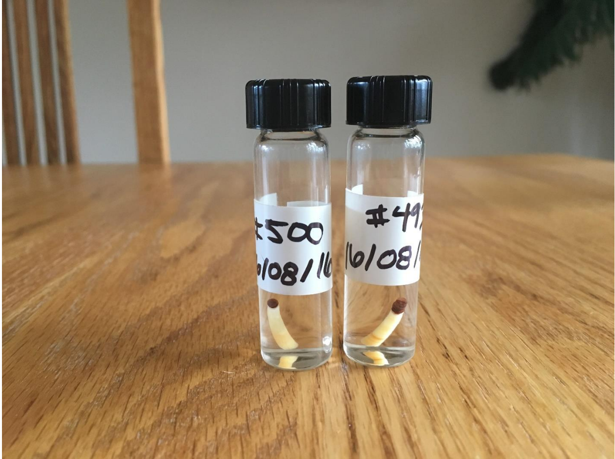
Figure 2.7. Microcore samples stored in 100% ethanol solution to prevent drying of cells (Image: Dana Harris, 2016).
