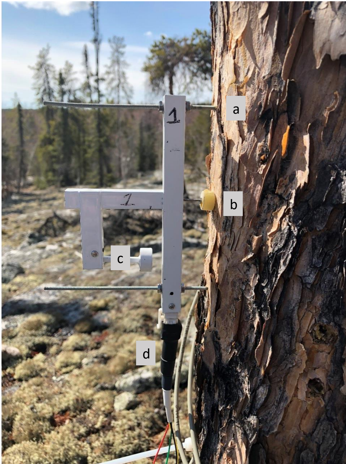
Figure 3.9. Automatic point dendrometer sensor fastened to tree at Treeville study site. (a) steel mounting rod; (b) sensing rod; (c) constant force cantilever; (d) LVDT cable connection. (Image: Dana Harris, 2018).
