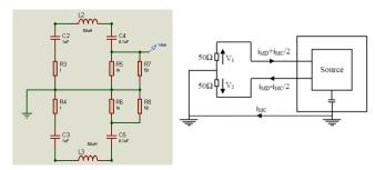
Figure 12. Conducted electromagnetic emissions measurement through the (a) LISN devise for both (b) common and differential modes.
