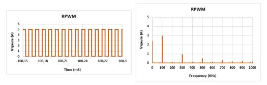
Figure 5. RPWM control signal: spectral analysis and signal characteristics.
