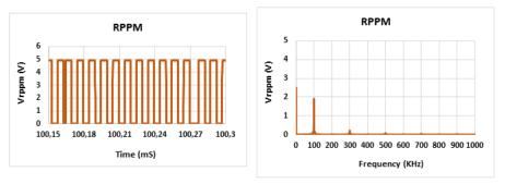
Figure 7. RPPM control signal: spectral analysis and signal characteristics.
