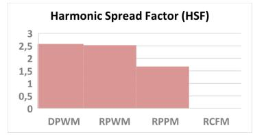
Figure 10. Analyzing the Harmonic Spread Factors for Modulation Techniques.
