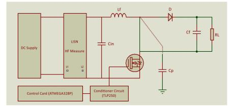
Figure 11. The Conducted Emissions Testing Framework for Boost Converter.
