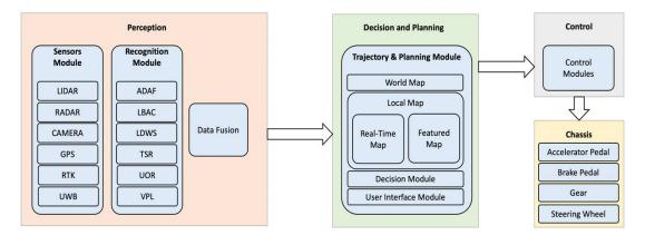
Figure 1. System Architecture for AVs [31].
