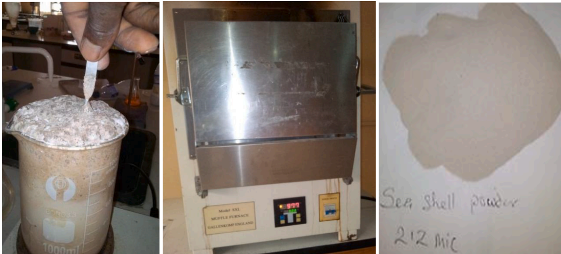
Fig. 2. Model SXL muffle furnace for preparation of African land giant and sea snail shell.
