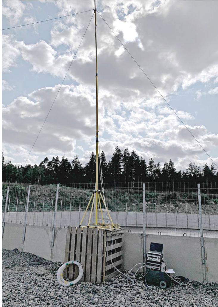
Figure 3. The measurement mast positioned downwind of the measurement site. The mast has four measurement points, the heights of which depend on the size and distance of the site. The suction hoses placed at the measuring points were connected to the photoacoustic analyzer.
