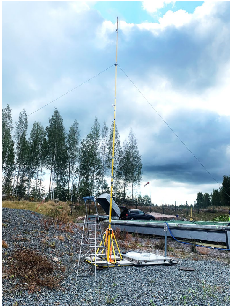
Figure 9. The measurement mast positioned downwind of the measurement site. The mast had four measurement points, the heights of which depend on the distance to the site.
