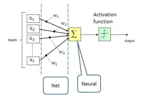
FIGURE 4.8: Artificial neural configuration [96].
