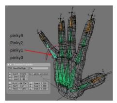
FIGURE 5.3: Illustration of IK applied to the base of the pinky – pinky1.
