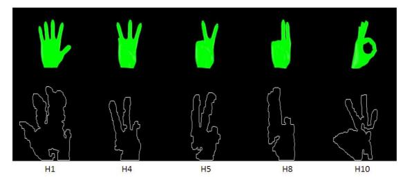
FIGURE 6.9: Examples of correctly recognised hand shapes from unclear and incomplete hand contour images on Background B.
