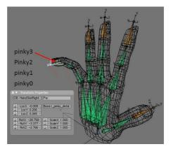
FIGURE 5.2: Illustration of IK applied to the tip of the pinky – pinky3.
