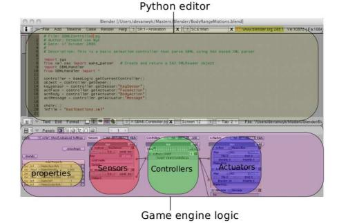
FIGURE 5.4: An example window configuration of Blender's Python editor and game engine logic [109].
