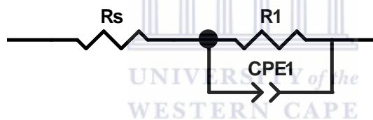
Figure 7.18: Equivalent circuit for neutral and p-doped PANI-PSSA electrode. R_s is the solution resistance, R_1 is the charge transfer resistance ( R_{ct} ), CPE1 denote constant-phase element.
