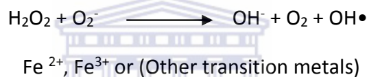
Figure 1.2: Hydroxyl radicals produced through a Fenton reaction using iron as the transition metal
