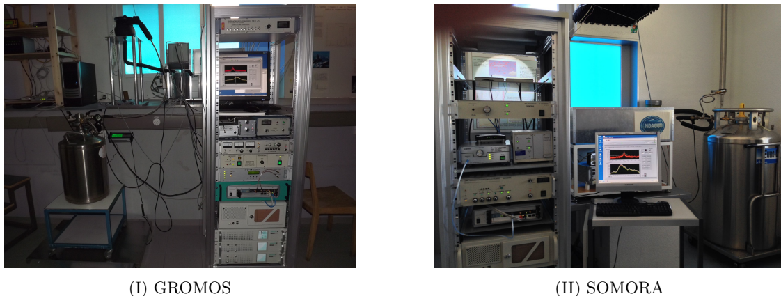
FIGURE 3.2: Pictures of GROMOS and SOMORA MWRs at the University of Bern (a) and at MeteoSwiss in Payerne (b). The two instruments are each in a temperature-controlled room and use a rotating mirror to constantly switch between the hot and cold calibration targets and the atmosphere. The atmospheric observations are done through a styrofoam window which is almost transparent for the incoming microwave radiation.
