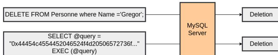
Figure 4.1: Two syntactically different MySQL queries performing the same operation on the system.
