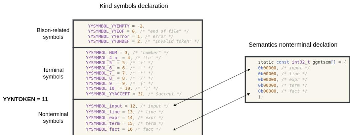
Figure 4.7: Example of the kind value attribution by Bison for a calculator grammar and the corresponding array of semantics generated by GAUR
