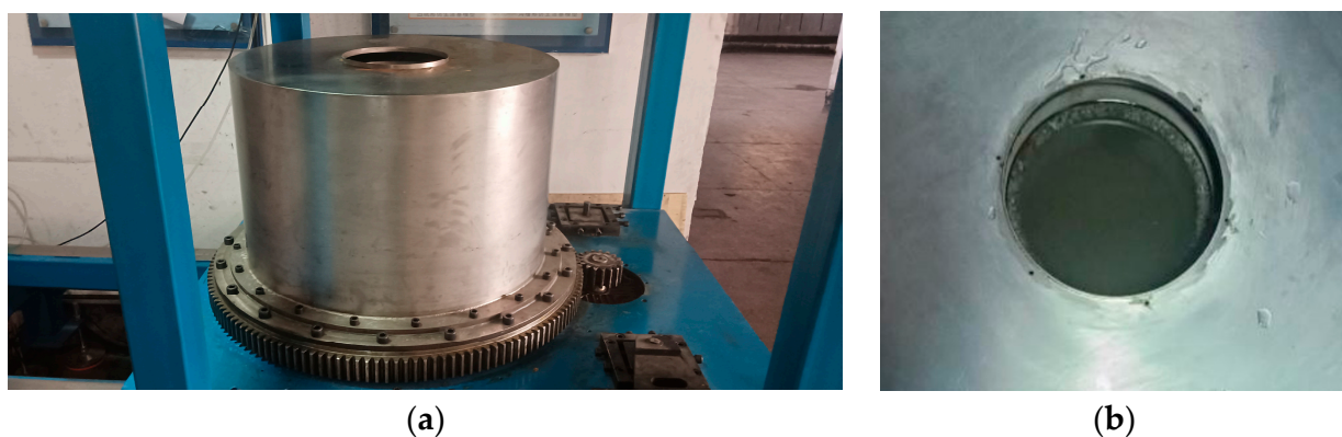
Figure 9. Abrasion test bench (a) Appearance of the test bench, (b) Wear parts installation.
