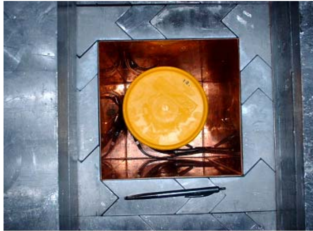
Figure 3.16: Top view picture of HPGe detector with the Marinelli beaker on top of it.
