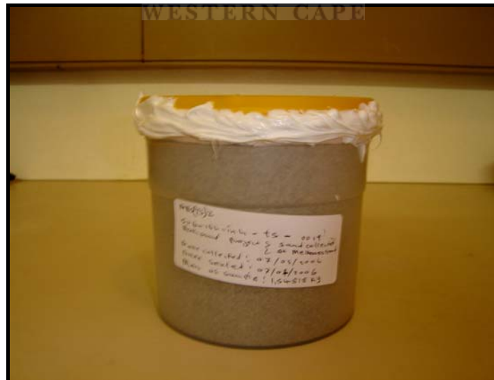
Figure 2.7: Picture of a sealed Marinelli beaker with a sample inside.
