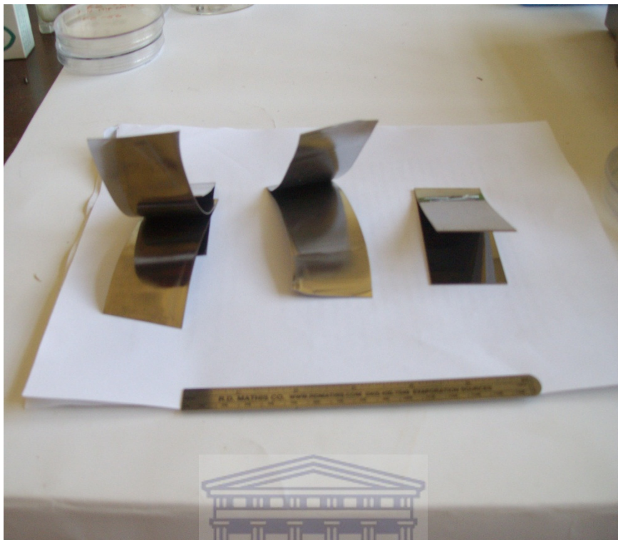
Figure 3.3: Polished stainless steel plates of an envelope type showing, from right to left, the shape deformation after several strikethrough in mills.
