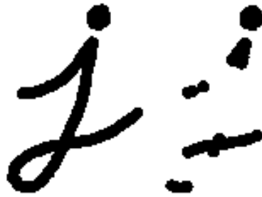
FIGURE 3.12: An illustration of the closing operator. Closed image (right) resulting from the original image (left).
