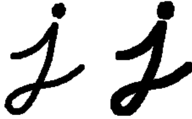
FIGURE 3.10: An illustration of the erosion operator. Eroded image (right) resulting from the original image (left).
