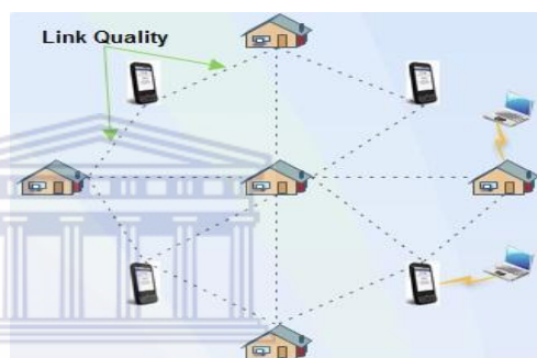
Fig. 1: A dynamic mesh network, applicable to a rural area, with static mesh routers inside homes, and mobile mesh nodes on cell phones. Note that link quality in such networks is continually changing as phones move around.
