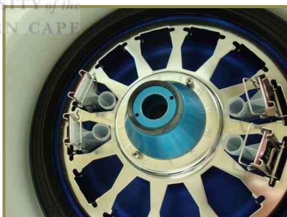
Fig 5. EZ Cytofunnel assembly loaded into Shandon Cytospin® 4 cytocentrifuge
