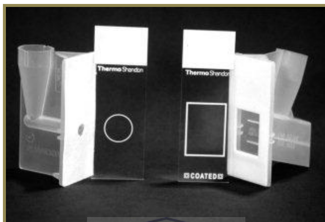
Fig 3. The EZ Cytofunnel (Left) produces a 28 \text{ mm}^2 circle of cells. The Megafunnel (Right) was developed to capture more cells ( 294 \text{ mm}^2 ). From Rosenthal et al. (2006).
